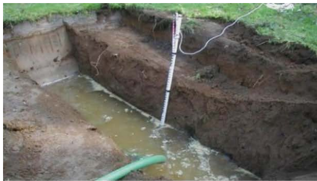
Pilot infiltration test (PIT)
