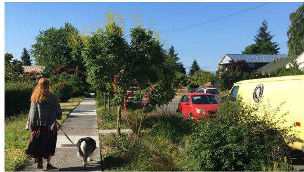
Cell with graded side slopes and underdrain, plants set back from edge of walk, Barton
