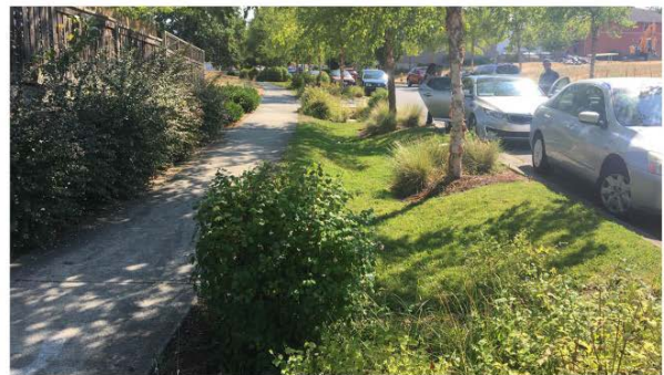
Cell with graded side slopes, grass is not approved due to subjective O&M, High Point
